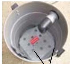
Upon receiving your vacuum system, lift off the lid. The protector plate should be located inside the can just below the HEPA bag.
